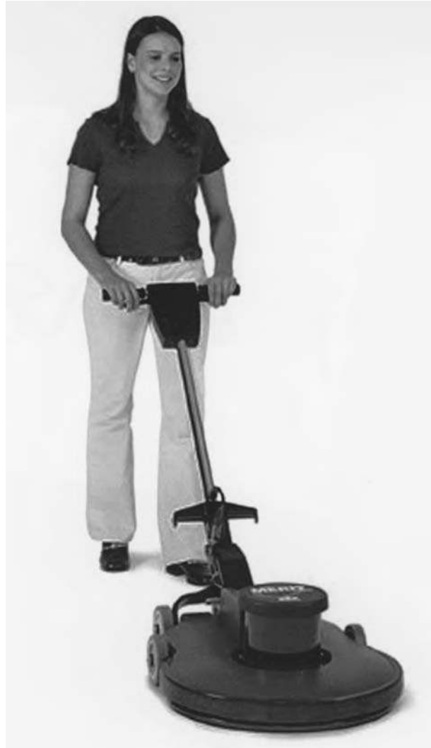
Figure 6-28 The Merit 2000 burnisher has a 2000 rpm speed and a “smart handle” that eliminates the need for a front wheel. It also contains a dust control system. (Photo courtesy of Windsor Industries, a Castle Rock Company, Englewood, Colorado.)
